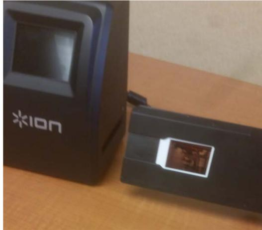
12. Turn off the scanner with the power button, unplug the USB cord from both the desktop and scanner, and remove SD card by gently pushing in and pulling out.
